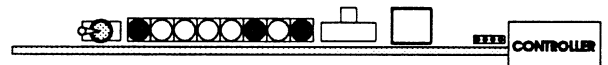
Fig. 5-22. Example: how to read the Automatic Memory Test results of a failure. In this case, bit 5 (0101) has failed.
